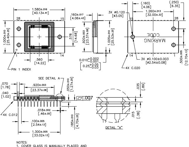
1. COVER GLASS IS MANUALLY PLACED AND VISUALLY ALIGNED OVER DIE – LOCATION ACCURACY IS NOT GUARANTEED.
