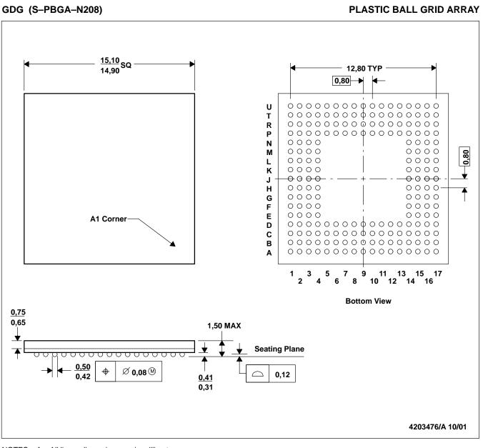
NOTES: A. All linear dimensions are in millimeters. B. This drawing is subject to change without notice.
