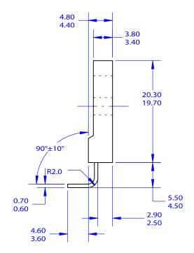
A. THIS PACKAGE DOES NOT CONFORM TO ANY STANDARDS. **B. ALL DIMENSIONS ARE IN MILLIMETERS.**
