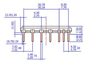
NOTES: UNLESS OTHERWISE SPECIFIED A) THIS PACKAGE DOES NOT COMPLY TO ANY CURRENT PACKAGING STANDARD B) ALL DIMENSIONS ARE IN MILLIMETERS C) DIMENSIONS ARE EXCLUSIVE OF BURRS, MOLD FLASH, AND TIE BAR EXTRUSIONS D) ( ) IS REFERENCE
