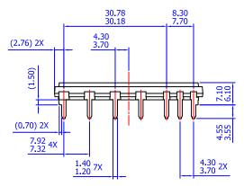
NOTES: UNLESS OTHERWISE SPECIFIED A) THIS PACKAGE DOES NOT COMPLY TO ANY CURRENT PACKAGING STANDARD B) ALL DIMENSIONS ARE IN MILLIMETERS C) DIMENSIONS ARE EXCLUSIVE OF BURRS, MOLD FLASH, AND TIE BAR EXTRUSIONS D) ( ) IS REFERENCE E) [ ] IS ASS'Y QUALITY
