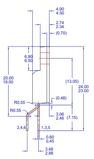
NOTES: UNLESS OTHERWISE SPECIFIED A) THIS PACKAGE DOES NOT COMPLY TO ANY CURRENT PACKAGING STANDARD. B) ALL DIMENSIONS ARE IN MILLIMETERS.
