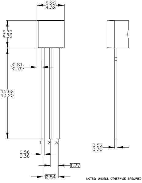
DRAWING WITH REFERENCE TO JEDEC TO-92 RECOMMENDATIONS. ALL DIMENSIONS ARE IN MILLIMETERS.
