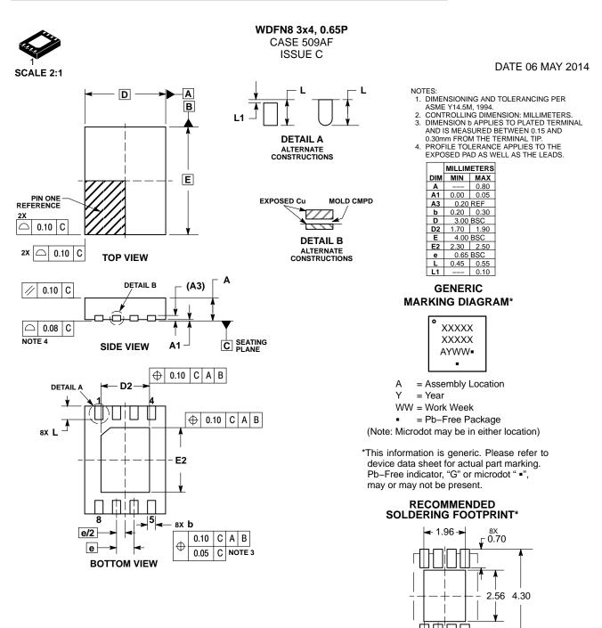
TUTUILITUIT 8X 0.65 → ← → ← 0.35 PITCH DIMENSIONS: MILLIMETERS
