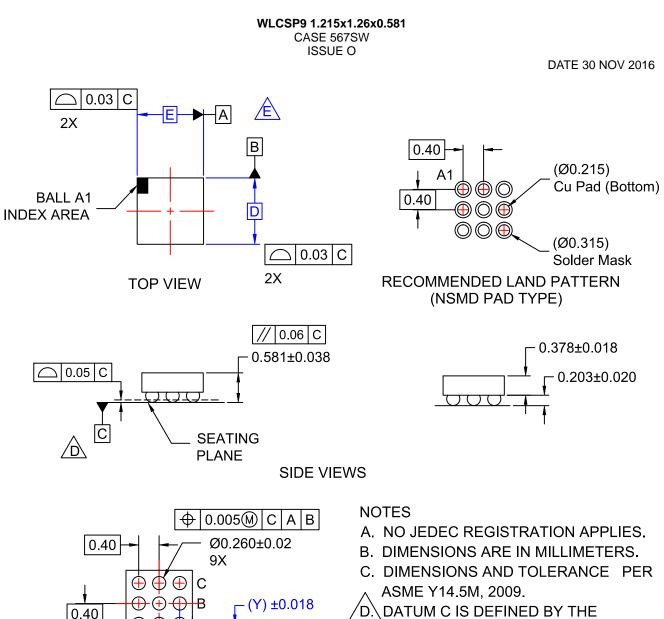
D. DATUM C IS DEFINED BY THE SPHERICAL CROWNS OF THE BALLS. E. FOR DIMENSIONS D,E,X, AND Y SEE PRODUCT DATASHEET.
