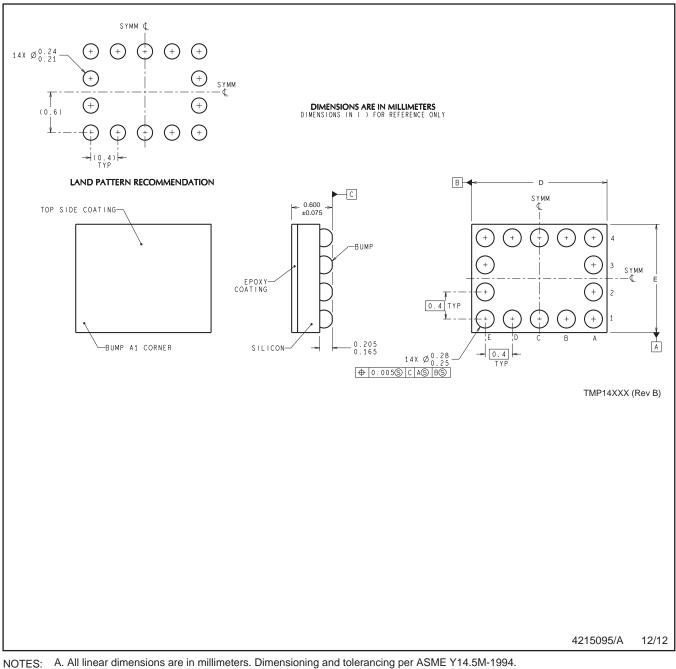
ES: A. All linear dimensions are in millimeters. Dimensioning and tolerancing per Al B. This drawing is subject to change without notice.
